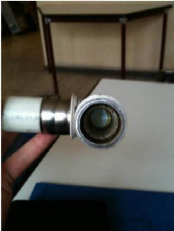
Above: condition of the pipe after 3 months of operation with AquaKat! The cooling system has now run perfectly since July 2009 and has not needed to be descaled since.
