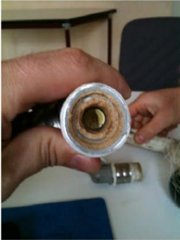
Above: condition of the pipe after approximately 3 months of operation
