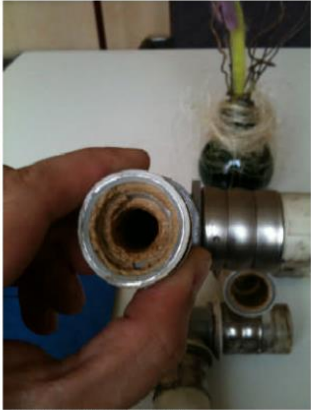
Above: condition of the pipe after approximately 3 months of operation
