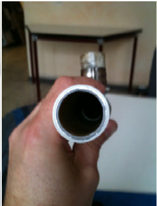
Above: condition of the pipe after 3 months of operation with AquaKat! The cooling system has now run perfectly since July 2009 and has not needed to be descaled since.
