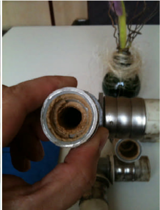
Above: condition of the pipe after approximately 3 months of operation
